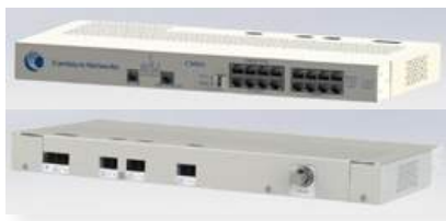
FIGURE 3. The Rack-Mounted Cluster Management Module 4
